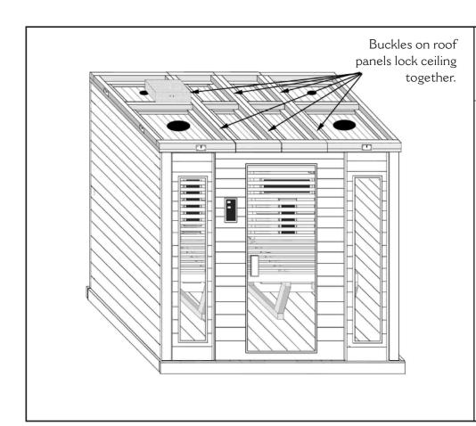
Buckle the three ceiling panels together with the four buckles located on the inside panel edges.
