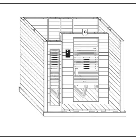
Insert door panel "G" into front base slot leaving a slight gap between wall panel. Cut securing strap on door panel and slide snugly against side panel.
