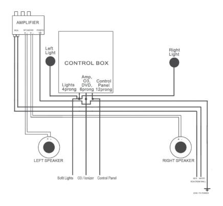
6 prong connection for Ionizer, Amplifier and optional DVD/LCD Power
