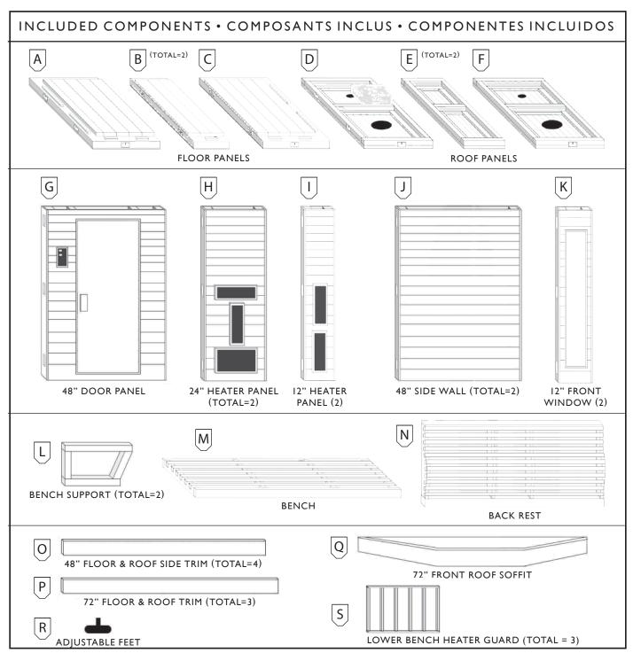
Before placing floor panels on ground, screw in adjustable feet "R" into each hole in bottom of floor panels.
